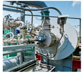
DUMAG® Industrial Burner IB4000GGS for 8 gases and liquids, 45 MW, Thermal Oxidizer for 22 Gas-/liquid streams
